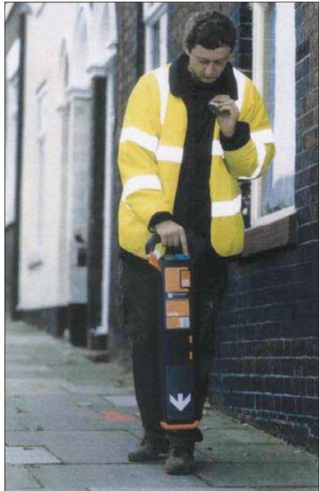
Figure 5 Using a cable locator
